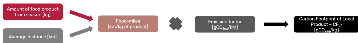
Figure 3: Scheme for the carbon footprint of local products assessment. Source: own elaboration based on Mancini et al., (2019) Producers’ and consumers’ perception of the sustainability of short food supply chains: The case of Parmigiano Reggiano PDO . Sustainability 11(3).
